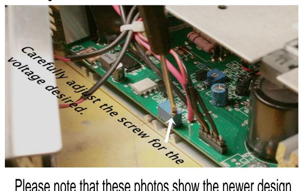
Please note that these photos show the newer design that has been in production for some time. This newer design has a top adjustment screw that is more precise. Re-assemble the unit by sliding the rear panel back into place and tightening the screws you loosened.
